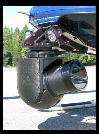
The C520 is the **smallest** and lightest system in the world to integrate all of the most popular digital cinema cameras. Cameras and lenses can be swapped out in less than 30 minutes, quicker than any other gyro-stabilized system on the market. The C520 does not have ITAR restrictions, and VectorSteering allows for look-down capability with no gimbal lock. No auxiliary junction unit is required and with in-flight calibration the C520 has an unbeatable horizon reference.
